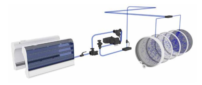
ADR FLUSHING in tank for internal cleaning with high pressure water jets fitted on the top of the tank. The jets are controlled by manual shutoff valves, and are supplied directly by the high pressure manifold.
